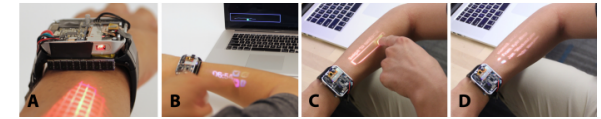
Figure 1. Our self-contained projection smartwatch (A) provides rectified graphics with touch input on the skin (B). We use a slide-unlock mechanism to reject inadvertent touches and provide a rapid projection calibration (C) before apps can be used (D).
