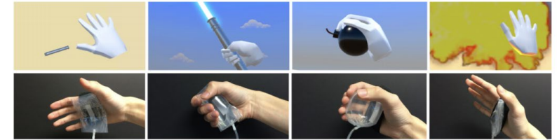
Figure 1. PuPoP is a wearable pneumatic shape-proxy interface for VR capable of popping up to primitive shapes and flattening on the palm. We demonstrate grasping emulation of picking up a virtual Lightsaber with a cylindrical PuPoP and throwing a virtual bomb with a spherical PuPoP.
