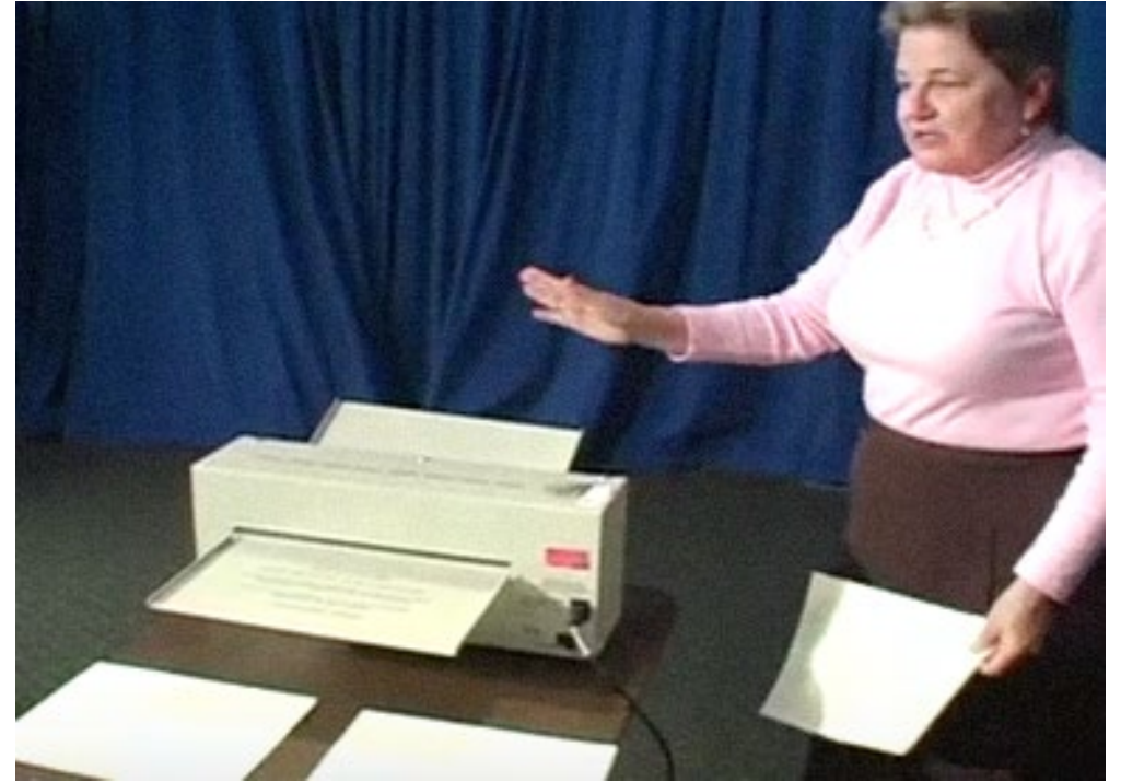
put in heater only black lines attract heat & swell
