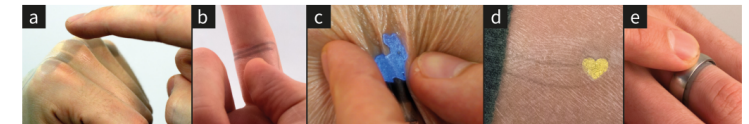
Figure 1: SkinMarks are conformal on-skin sensors and displays. They enable interaction on five types of body landmarks: (a) skeletal landmarks, (b) skin microstructures, (c) elastic landmarks, and (e) accessories.
